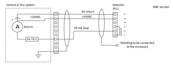
In this case, the output current is not isolated from power supply, consumed by the detector.
