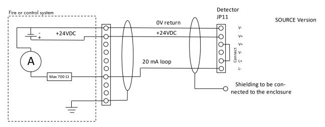
In this case, the output current is not isolated from power supply, provided from detector (standard connection).
