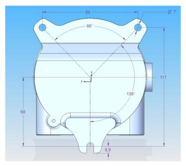
Drilling dimensions for support fixing.
