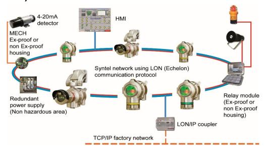
In this network version, an electronic board is inserted in the detector body and is used for electric connection.
