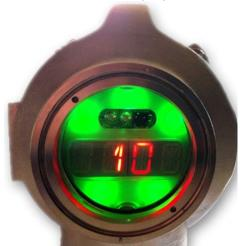
The orientation enables a communication with an  $\frac{1}{2}$  horizontal angle about 35°, an  $\frac{1}{2}$  vertical-up angle about 30° and a vertical-down angle about 50°.
