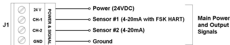
Figure A - 6 Power and Signal Connector J1 on HART Supported iTRANS-2
