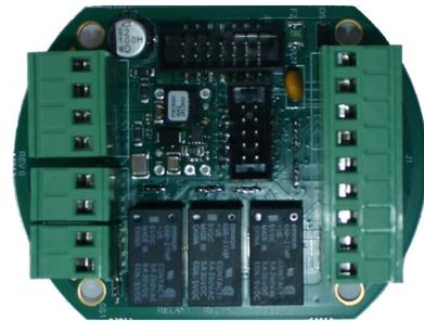
Figura A - 1 **iTRANS-2** Tablero HART
